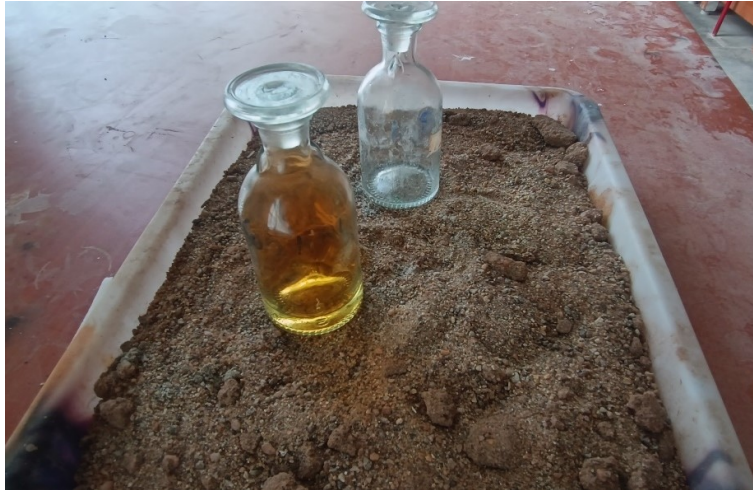
Fig.21. Storage of concentrated acid in sand base.
